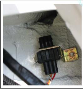
contacts might be a good idea cap, and would require a custom bracket to mount the connector. If this method is used, gold plated place of the 3-pin socket. Because it is located in the engine compartment, it should be protected by a To enable the car to be used only with standard 16-pin interfaces, a DLC connector could be spliced in
